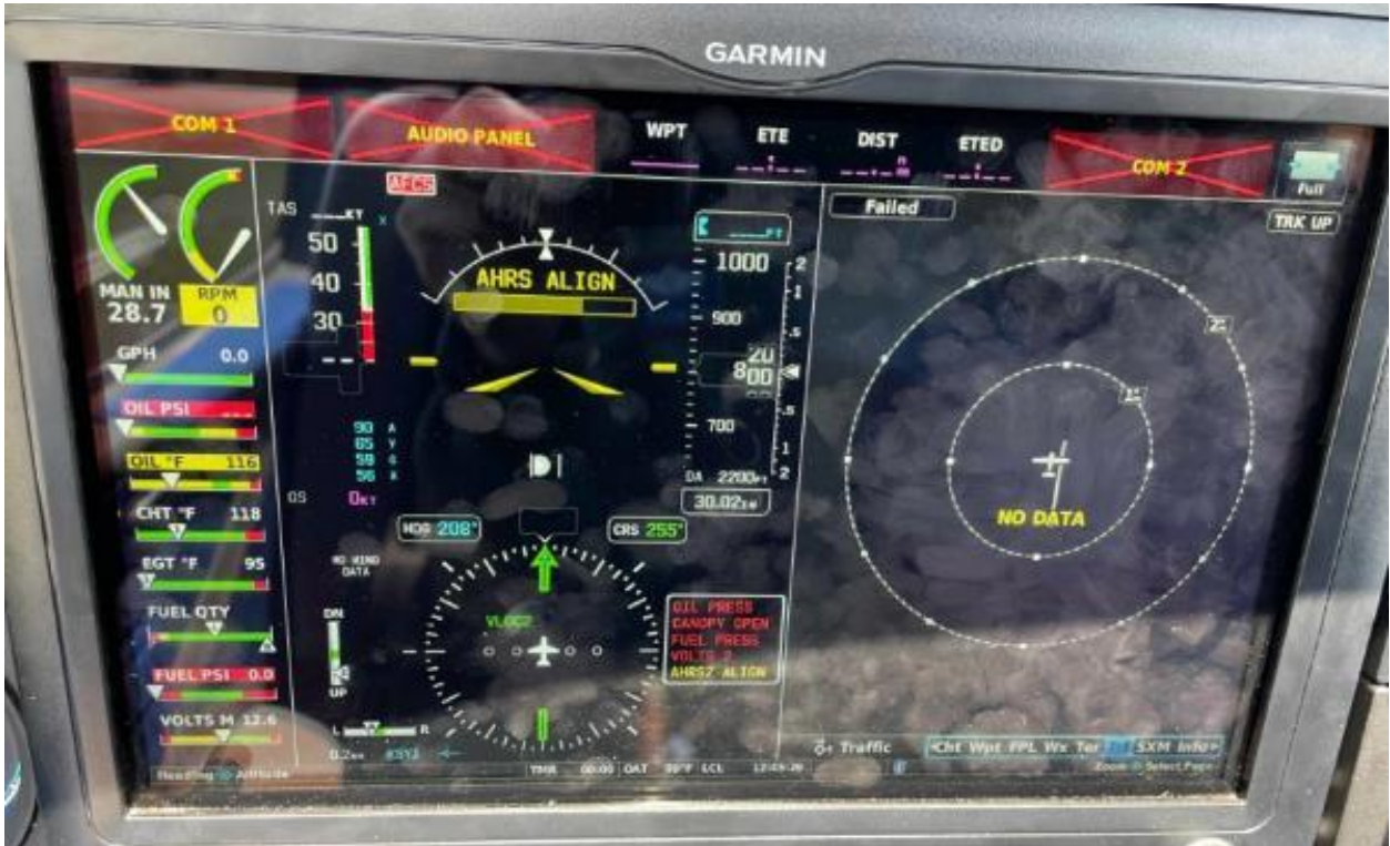
Garmin G3 Primary Flight Display with Power Displays on startup.
