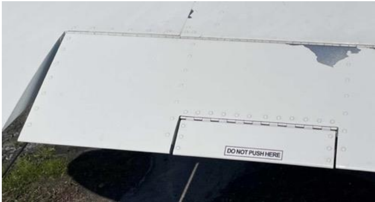
Electrically actuated aileron trim tab.
