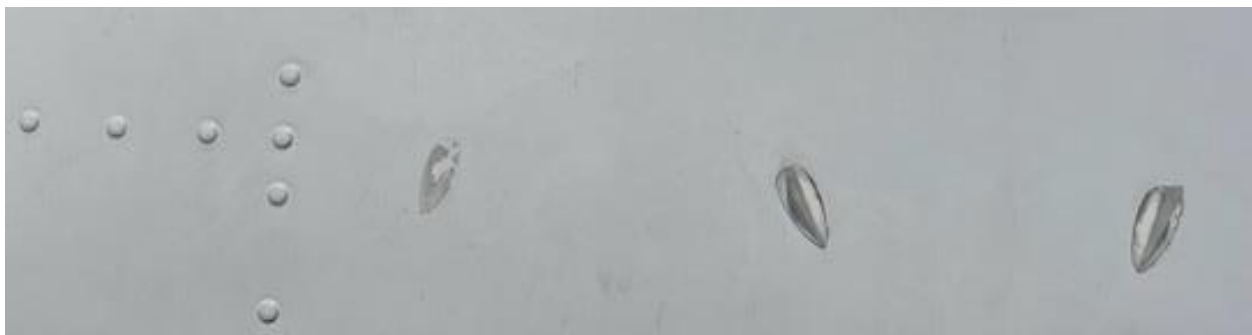
Adhesive mounted vortex generators. (One's missing. So how many do we need???)
