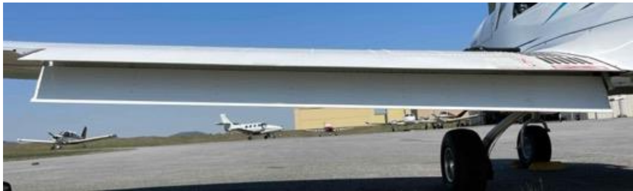
Split flaps under the trailing edges.
