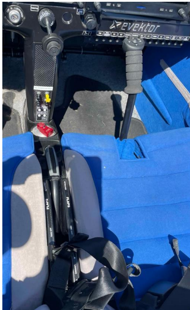
Harmony center Power quadrant and manual flap lever.
