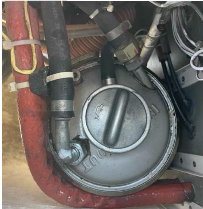
Rotax oil filler cap. (Where's the dipstick?)
