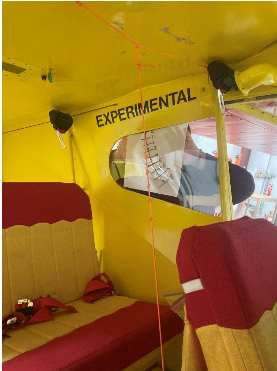
Figure 7. Flap Position Theodolite
