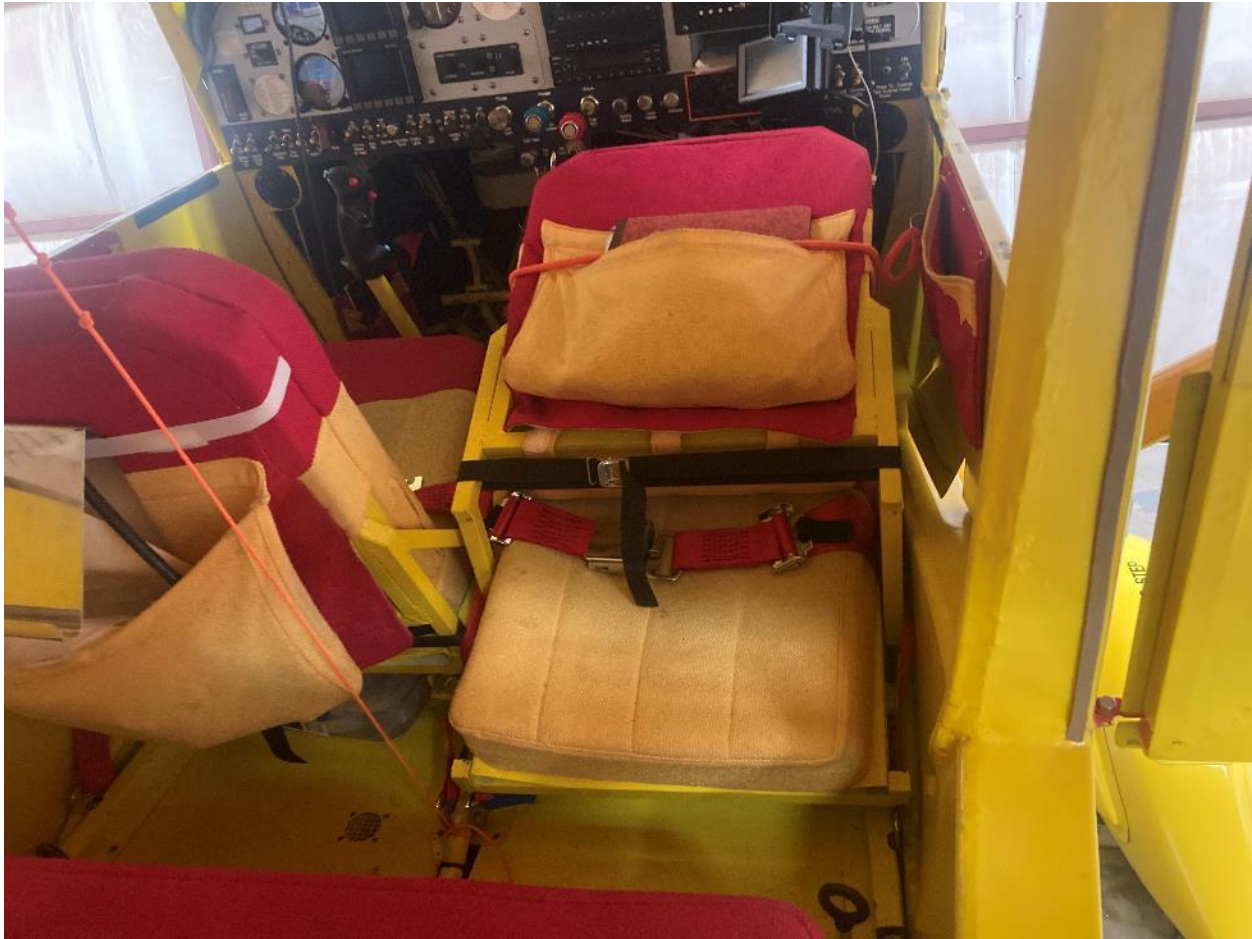
Figure 8. Right Front Seat folded forward to make room for data sighting
